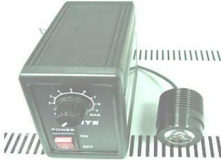
Figure 3. The developed stroboscopic LED light module
